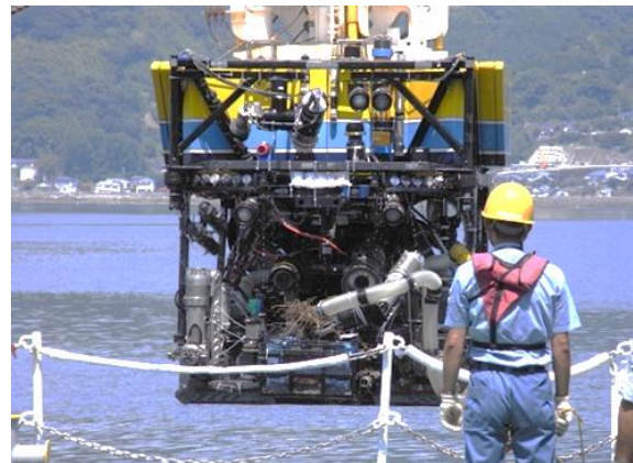
Fig.28 The new ROV "Hyper-dolphin" for heavy work which can be evaded to 4500m
