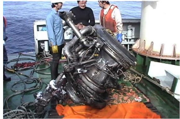
Fig.27 The main engine drawn by ROV up on the board
